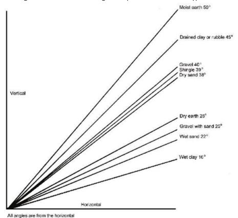
It can be seen from the above diagram that even shallow trenches can collapse depending on the soil type
