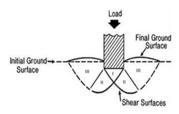
The figure represents a foundation (hatched) sitting on horizontal ground equal in level on both sides. The foundation is loaded and the three zones marked I,II & III are what Terzaghi suggested to be the soil wedges 'mobilised' by the loading.
