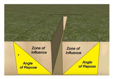
In basic terms, a competent person should examine the soil being excavated to determine what type of soil it is and how long it will "stand-up" under its own weight. Soil conditions, including soil type and ground water levels, are two critical factors effecting the type of trench hazard(s) and choices of protective systems.
